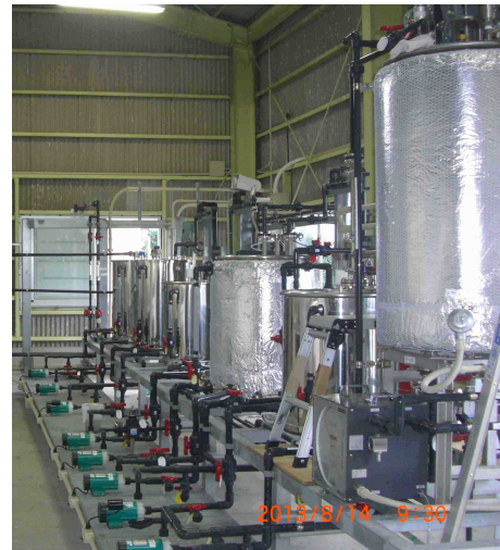
Photo 1. Small pilot plant set at Itoman city in Okinawa. The top tank is the fermenter with 200L volume.
